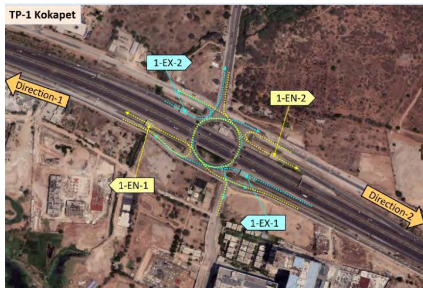
Figure 2-5 : Rotary Type Interchange with 4 toll booths.
