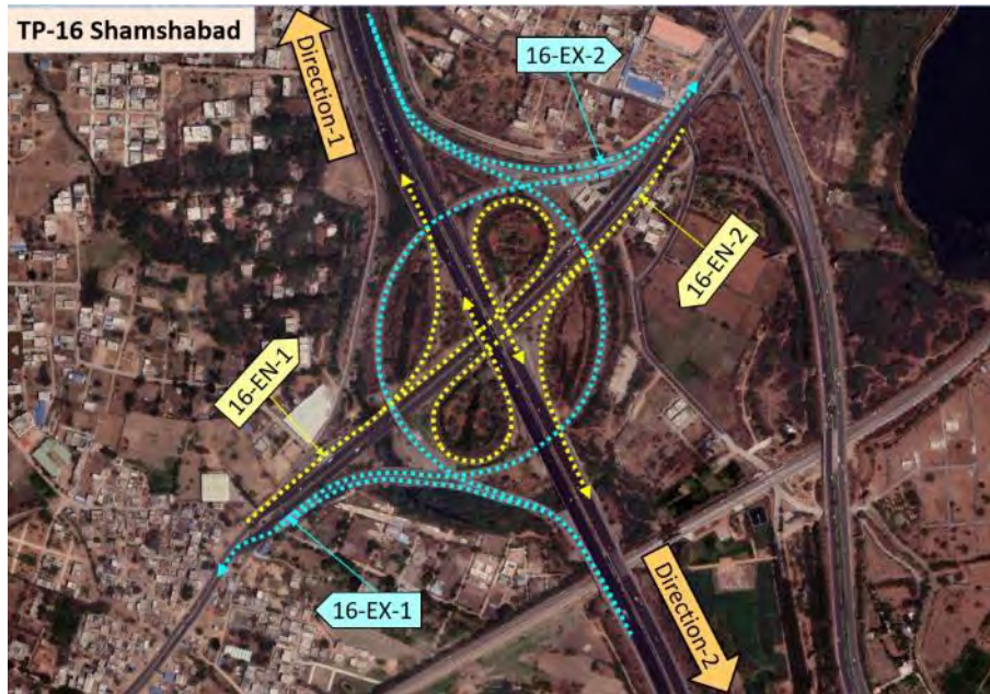
Figure 2-8 : Shamshabad Interchange and Ramps
