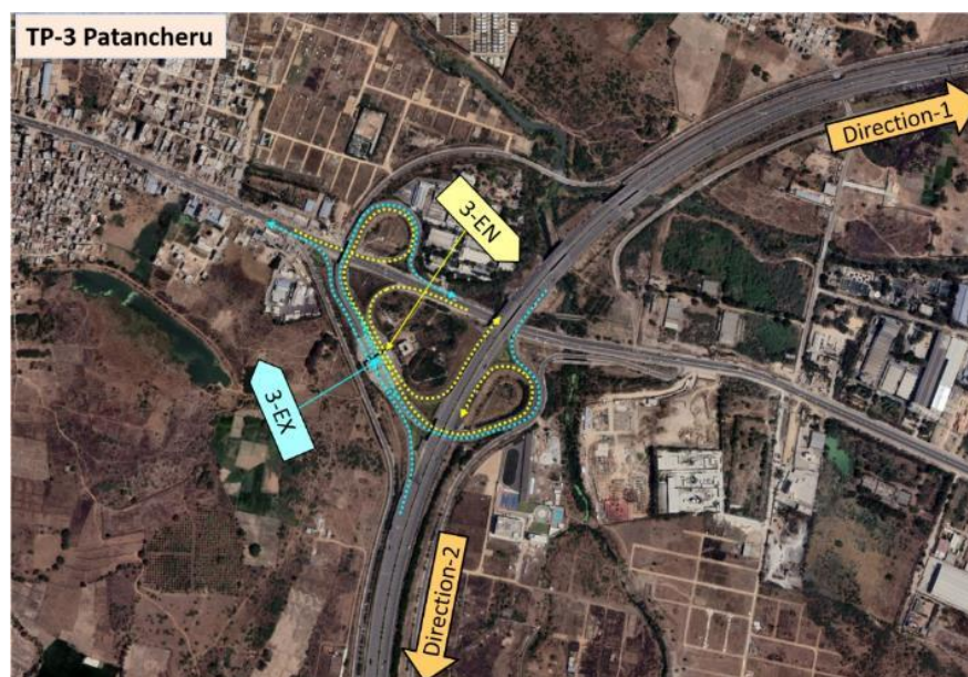
Figure 2-7 : Double Trumpet Type Interchange
