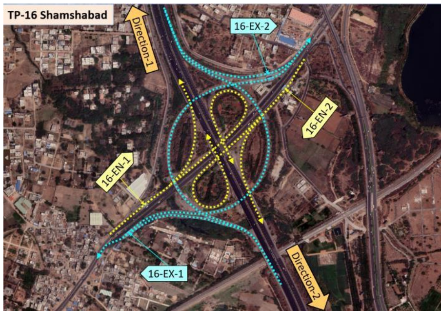
Figure 2-8 : Shamshabad Interchange and Ramps
